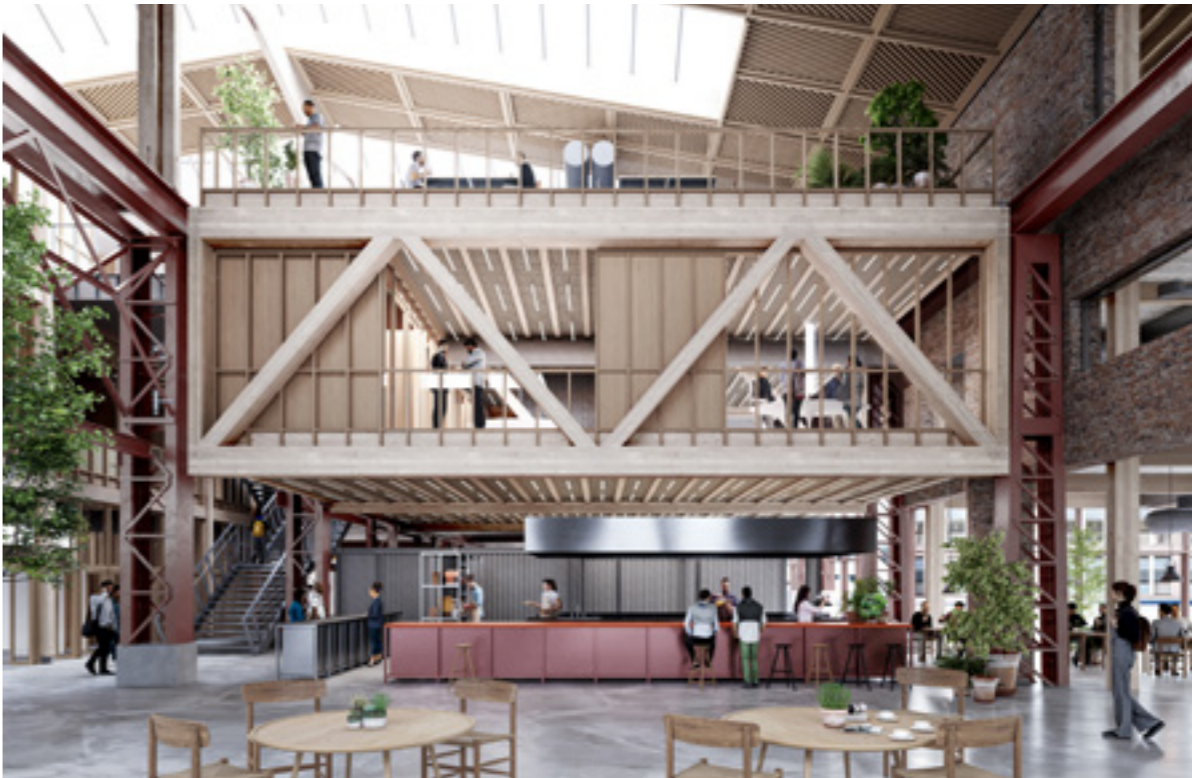
The added timber structure is suspended from the existing steel frame, creating a sequence of spaces with vertical connections between floors and activities.
